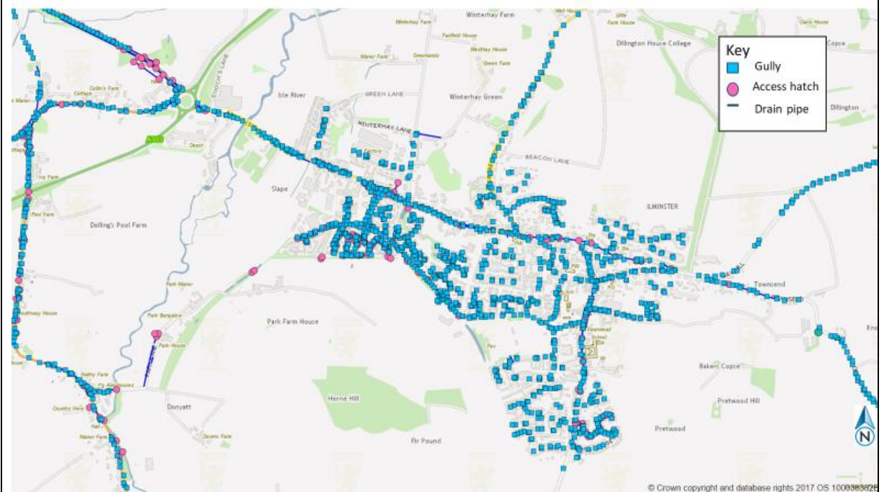
Figure 18: Highways gullies in Ilminster
